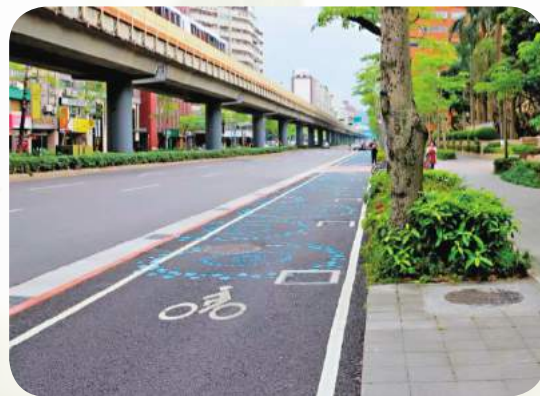
▲ Permeable pavement on bike lanes
